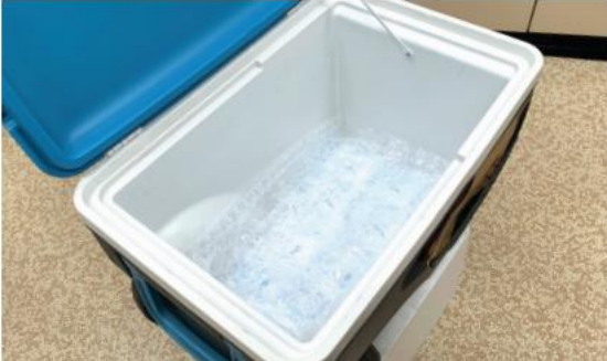
Figure 3: Insulating material placed in bottom of cooler
